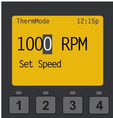
Setting Thermal Mode Pump Speed
