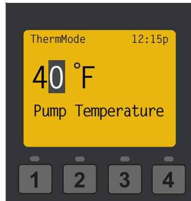
Setting Thermal Mode Pump Temperature
