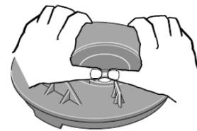
Press Seal into plate firmly
