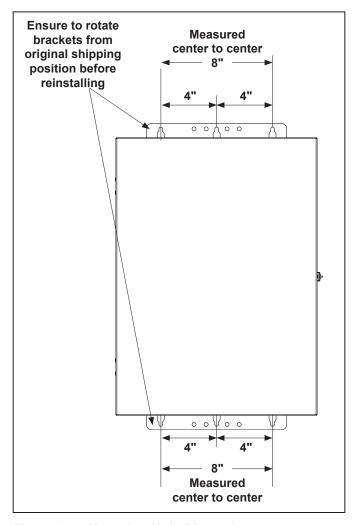
Figure 3. **Mounting Hole Dimensions**
