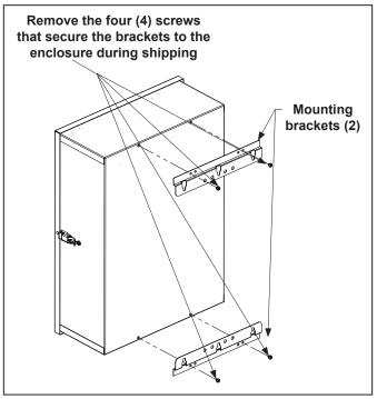
Figure 1. Enclosure Installation
